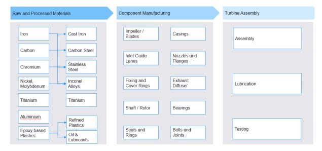
Source: Global Value Chain and Manufacturing Analysis on Power Plant Turbines, NREL Note: Examples in the raw and processed materials, components and turbine assembly are not exhaustive
