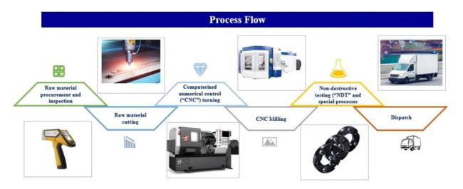
Brief details of our "make to print" manufacturing process which includes relevant testing activities at various stages is set out below:
